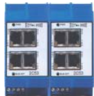
Two 2C53 Ethernet Switches
