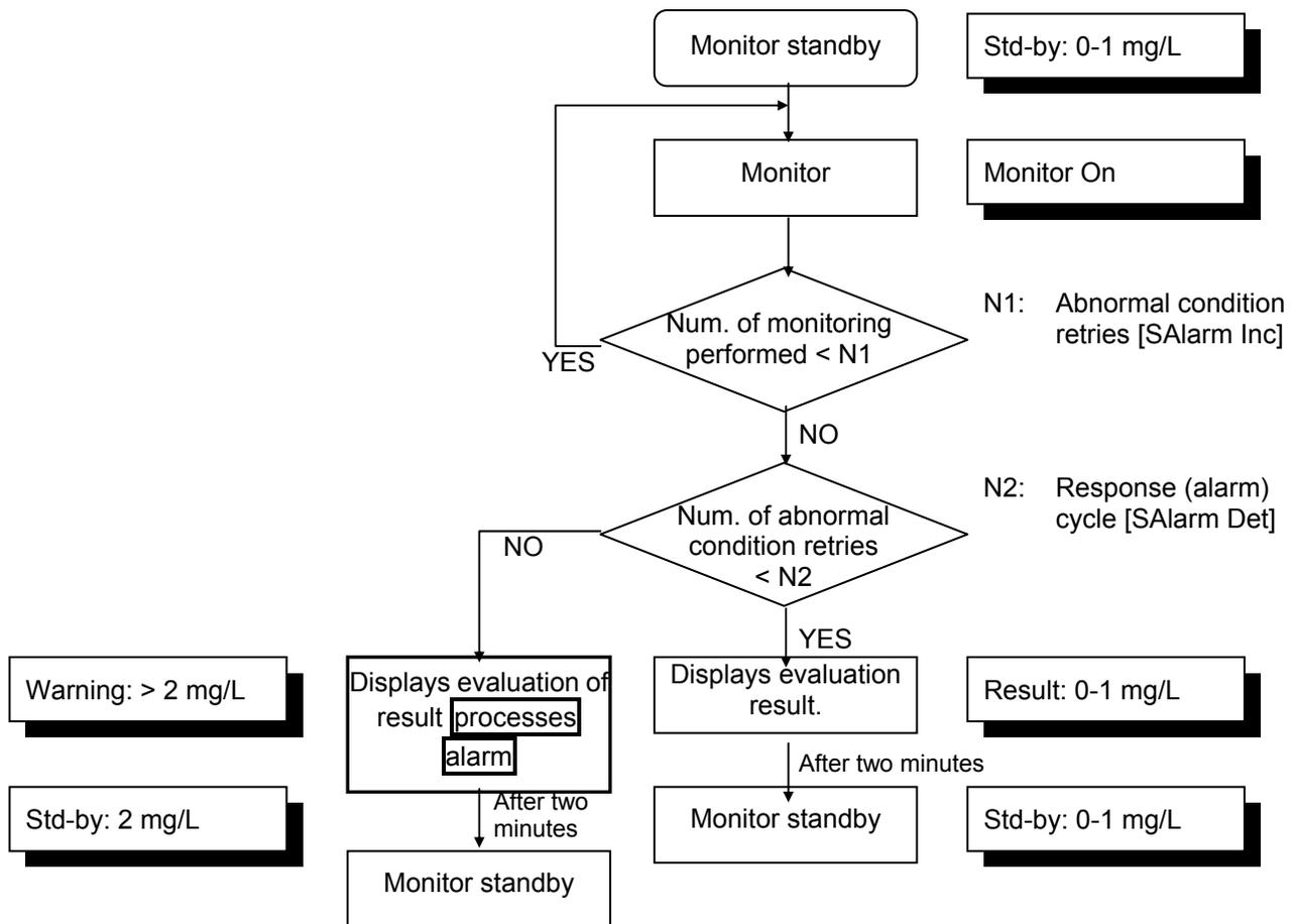
[3] If an abnormal condition occurs repeatedly in a series of automatic monitoring at Monitor interval [SIntvl], or in manually initiated monitoring, the abnormal-condition alarm will stay on continuously.
