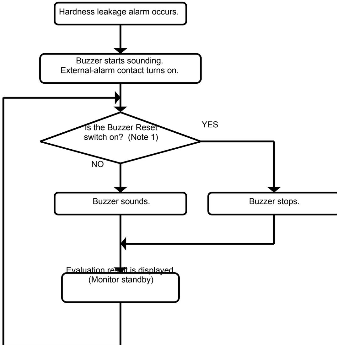
Note 1: The Buzzer Reset switch also functions as a manual monitor switch.
