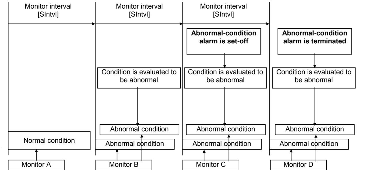
Monitor A: The result is below the alarm set point (setting), and therefore the condition is deemed to be normal.
