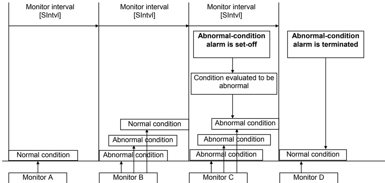
Monitor A: The result is below the alarm set point (setting), and therefore the condition is considered normal.
