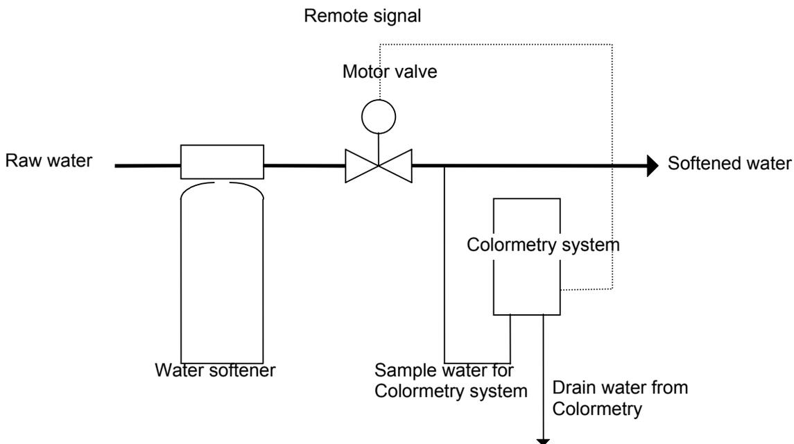
To prevent such a problem, select Remote signal delay time [SRte Sgl dl] setting and ensure the required pressure (7.1 ~ 71 psi) at the Colormetry inlet (0 ~ 30 seconds).
