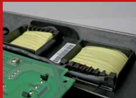
Built-in DC-link reactors reduce harmonic noise and protect the drive. Integrated EMC filters are also available to minimize RFI interference (meets EN 55011 A2, A1 or B).
