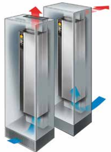
Back-channel cooling: A smart, dedicated kit allows chassis/IP00 enclosures to be mounted in Rittal cabinets so cool air removes 85% of excess heat without contact with the electronics.
