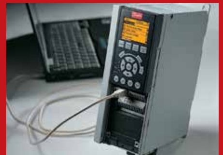
The VLT® AQUA Drive can be remotely commissioned and monitored through a USB-pluggable cable using MCT 10 setup software.
